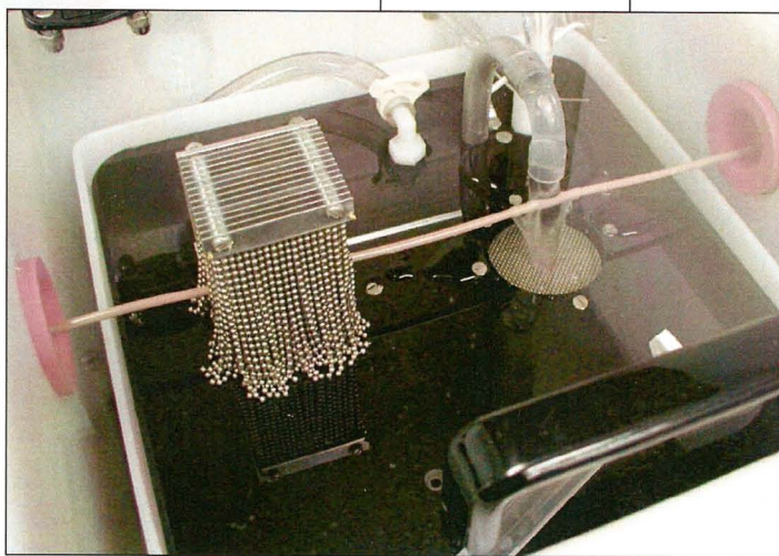
Bead chain shown for water removal. The bead chain may be removed when mechanical contact with the product is prohibited.
